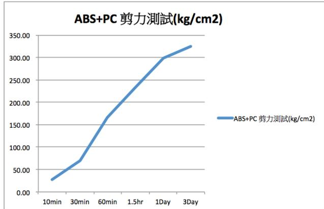
\*試驗方法: 參考ASTM D1002 - 05 Standard Test Method for Apparent Shear Strength of Single-Lap- Joint Adhesively Bonded Metal Specimens ! by Tension Loading .! \* kgf/ cm<sup>2</sup> 換算成 kg/cm<sup>2</sup>須乘上9.8。
